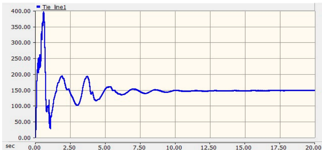
Figure 14. Damping Oscillation using ANN Controller under Load Condition 1734 [MW].
